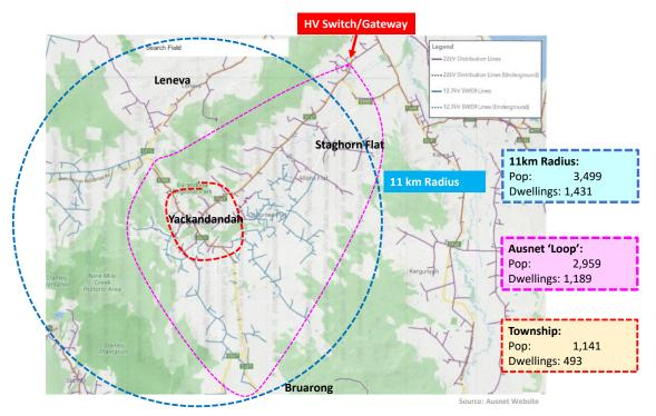
The map shows (in red) the location of the HV switch at Patrice Vale. This switch is where all AusNet data for imported electricity into the Yackandandah Valley was taken, feeding into the various 22kV and 12.7kV SWER distribution lines (also shown on the map).
